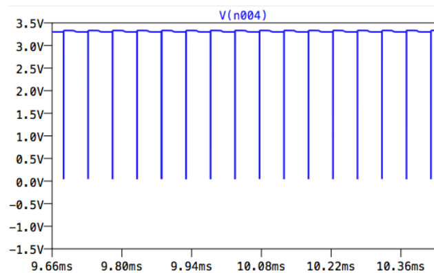
Figure 8: MOSFET output voltage waveform from the LT Spice simulation
