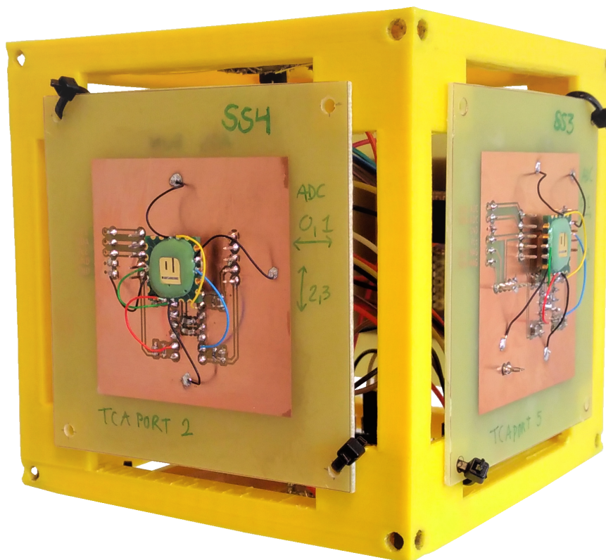
Figure 10: The CubeSat mock-up. Two of the sun sensor panels can be seen.
