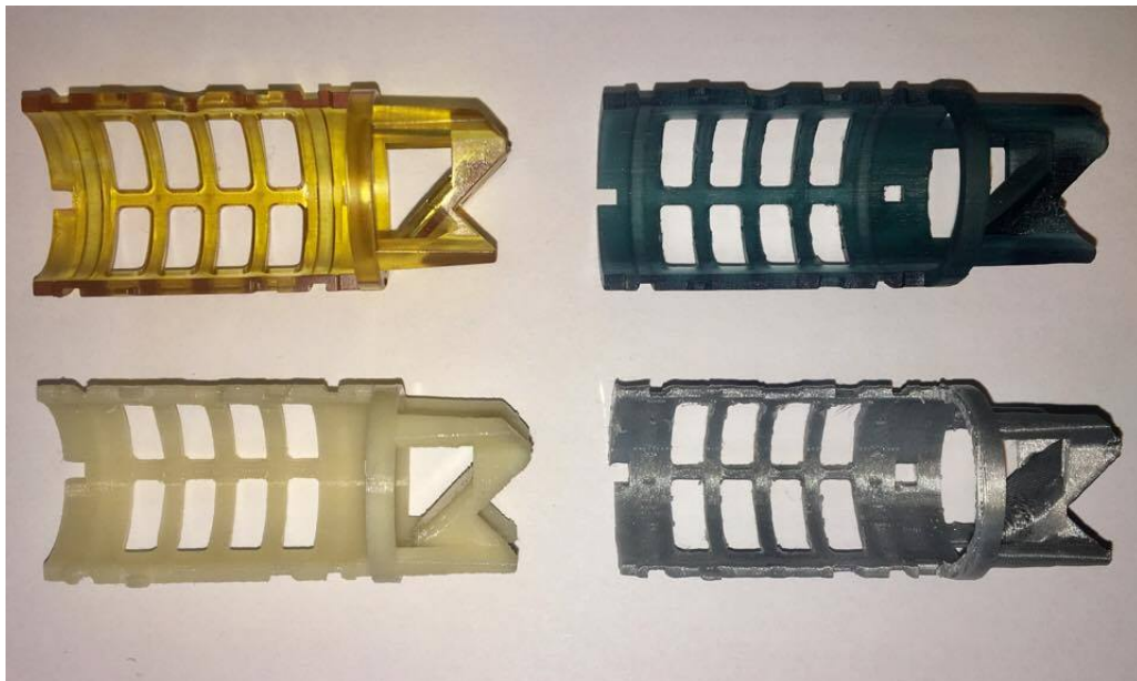
Figure 3.3: Yellow: Original Flow Meter. Blue: High Quality 3D print from FormLabs 2. White: 3D print from Afinia H800. Silver: 3D print from Ultimaker2+.
