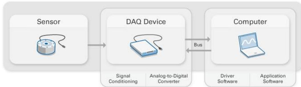
Figure 17. DAQ chain example. Source: [54]
