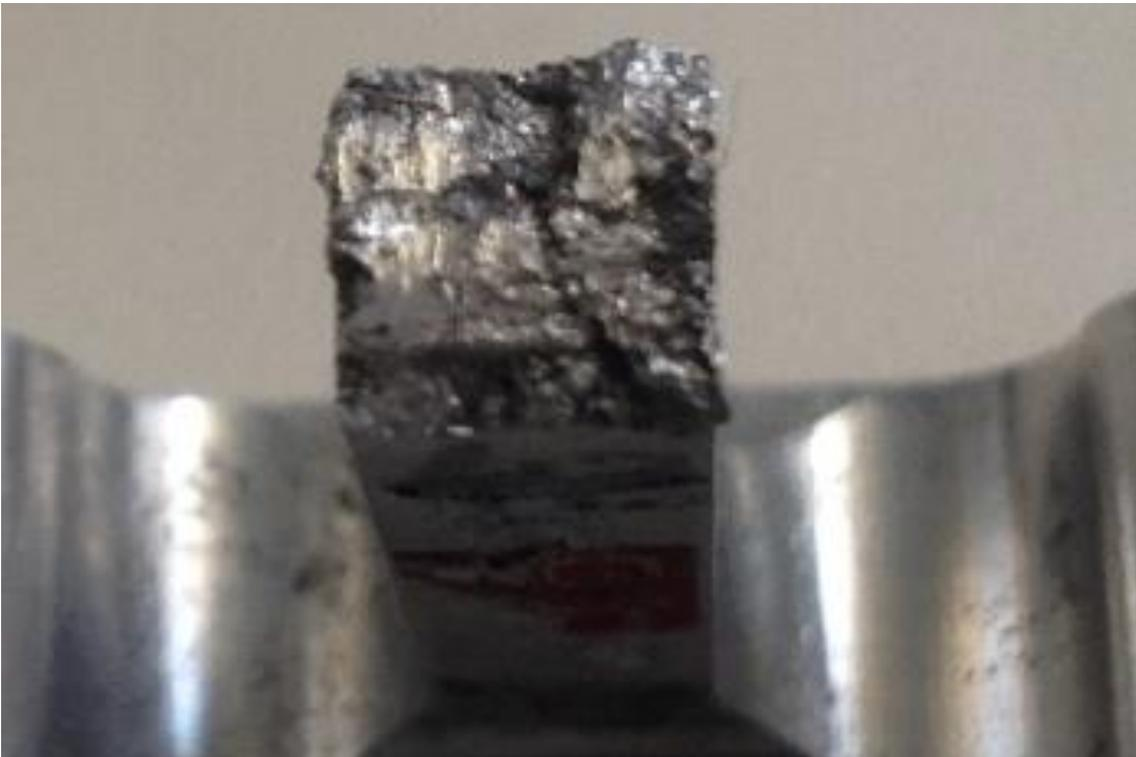
Figure 53. Sudden fragile fracture detail.
