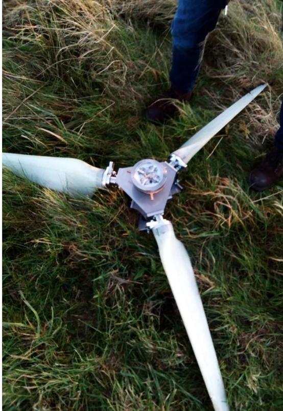
Figure 50. SWT rotor after fatigue break
