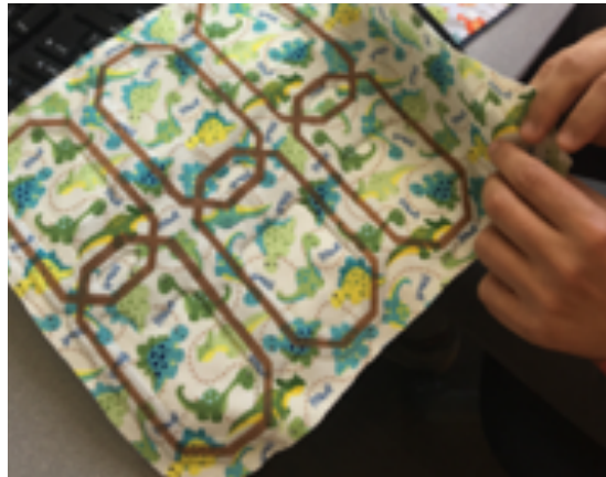
Figure 17 Printed (flexible) MRI coils (prototype)
